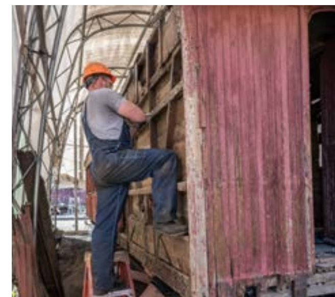
Cody Cartwright, Carpenter, removing siding from baggage end of the 211. > Photo by Jerry Day
